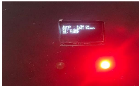
Figure 8. LCD Display with Input Gate Closed and Output Gate Closed
