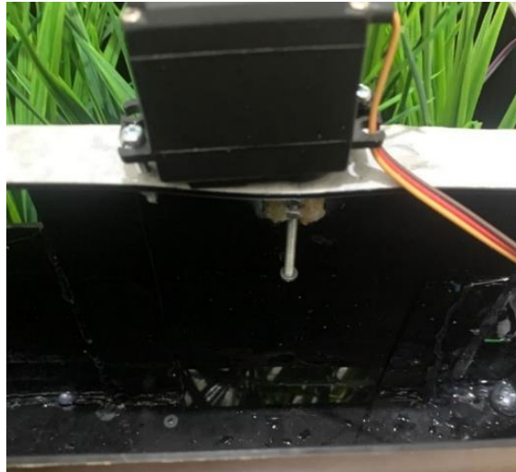
Figure 12 Output Gate in Open Position
